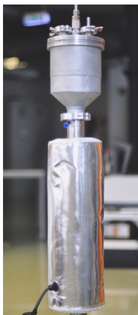
WSR50 with a diffuser diameter of 50 mm for the multigram scale
